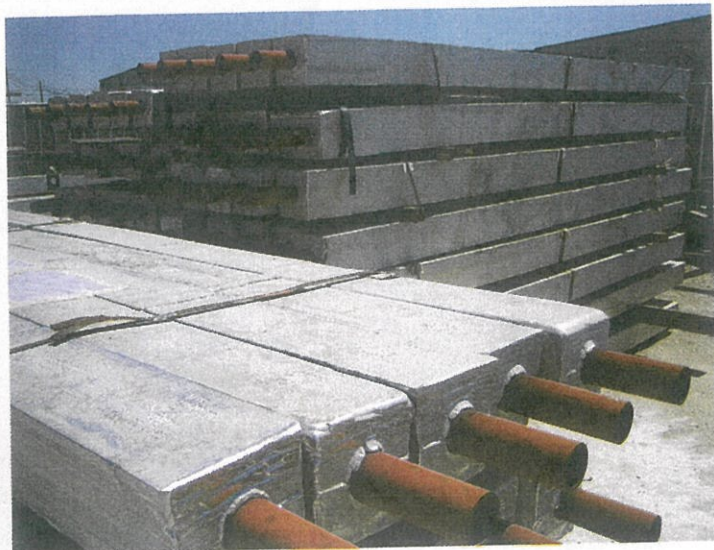
FIGURE 9.5.8 These aluminium sacrificial anodes are attached to the underwater steel structures of offshore gas platforms to protect them against corrosion.
