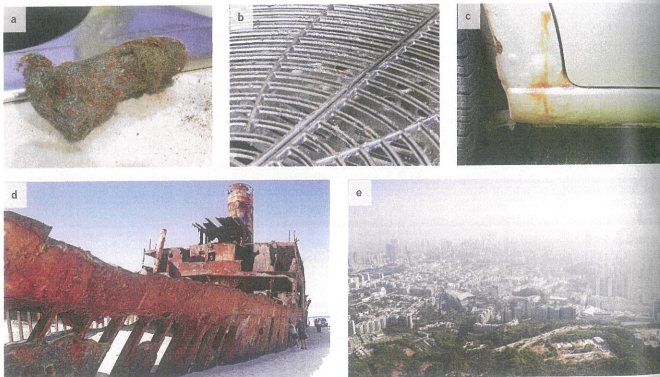
FIGURE 9.5.3 Wet corrosion. (a) A piece of steel wool (iron) does not corrode on supermarket shelves. However, once it becomes wet through use, it corrodes quickly. (b) An iron barbecue grill that has been coated with grease shows little sign of corrosion, even after being exposed to the rain for some time. (c) Rust in a car generally starts inside door frames, under mudguards, or in places where the paint has been chipped. (d) Shipwrecks corrode rapidly and will eventually disintegrate. (e) Corrosion occurs more rapidly in cities with a pollution problem, particularly where the pollutants include acidic oxides such as nitrogen dioxide and sulfur dioxide.
